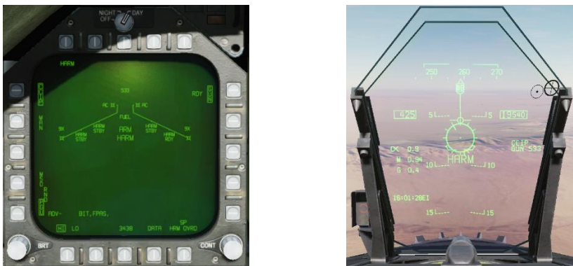
Figure 206. "HARM" displayed on Stores page and HUD.
