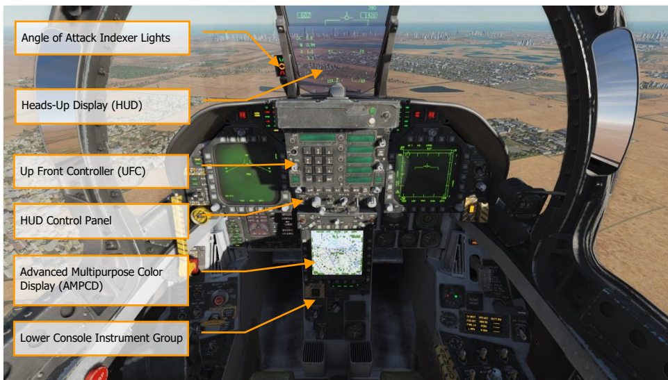
Figure 5. Center Instrument Panel
